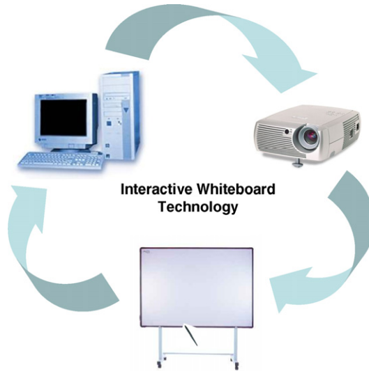
Fig. 1. How IWB technology works. The computer images are displayed on the board by the digital projector. The images then can be seen and all applications on the computer can be controlled via touching the board, either with your finger, or with an electronic pen/stylus.
